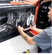
This is what the manual window regulator and scissor assembly look like once extricated from the door shell.
