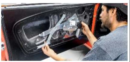
As you can see in this photo, the more compact Electric-Life power unit installs with the factory mounting holes for the scissor assembly and includes a new guide track. While you don't have to remove the door glass for installation, we were replacing the door glass belt line moldings and opted to pull the glass out for more room.
