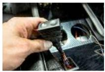
Switches can be mounted in the door, in an OE console, or just about anywhere. (Lots of photo ideas online. Let Google help you there.) Since our Mustangs to Fear console was ordered with the optional power window switch openings, that is what we used. Route the wiring as needed, secure your switched power and ground, insert the wired terminals into the switch connector cavities, and then snap the switches into place.
