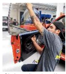
■ Tighten the power regulator mounting nuts and then reinstall the glass if removed. If you need to power the regulator to line up the window rollers and the glass' track, use a 12-volt power source to power the motor up or down to get things in line.
