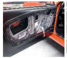
Begin by removing the door panels to access the regulator mounting bolts. You'll have four bolts to remove the regulator itself and several more to remove the scissor assembly on the '65-'66.
